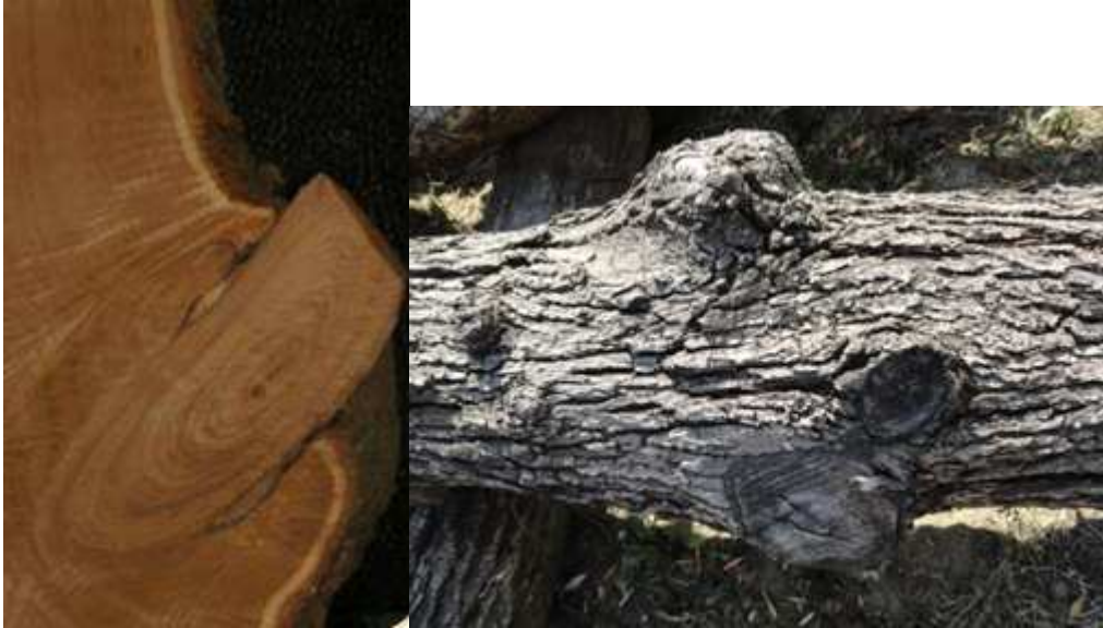
Figura 118: Nós (Fonte: http://www.pannonpower.hu/en/biomass/wood-defects ).
